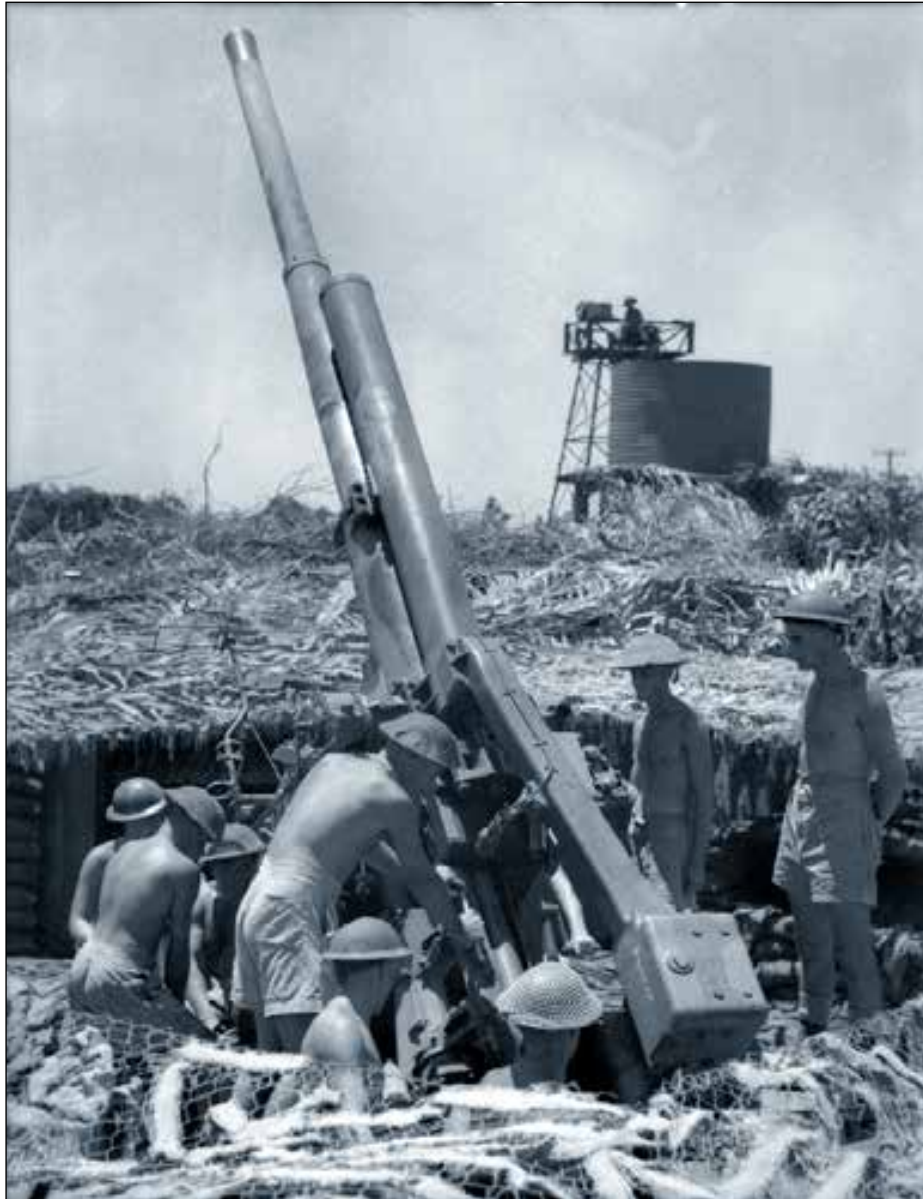
A gun crew of 14th Heavy Anti-Aircraft Battery, loading at Darwin in November 1942. The 3.7-inch gun, of the type used here, was the mainstay of anti-aircraft defence in Australia. In the background is a spotting tower. (AWM 027793)
