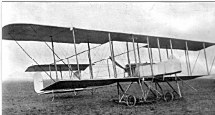
Maurice Farman (Shorthorn). Engine - 70h.p. Renault. Cruising speed - 45 mph. A specimen of the authors first machine
