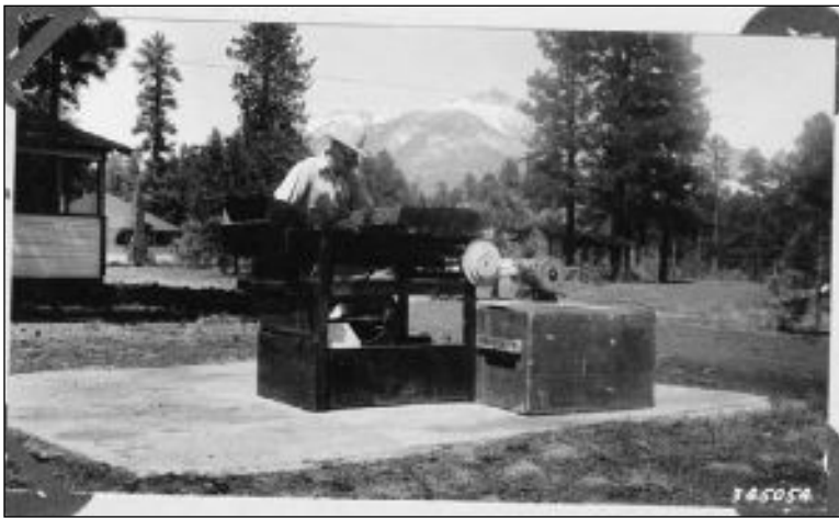
Figure 4. "Clipper" fanning mill for cleaning tree seed before planting at the Little Leroux Springs nursery. Photo taken at FVEF by Roland Rotty in May 1937. USFS photo 345054.
