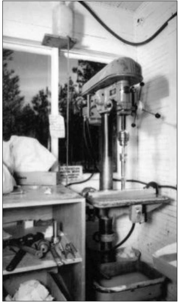
Figure 6. Core cutting equipment.
