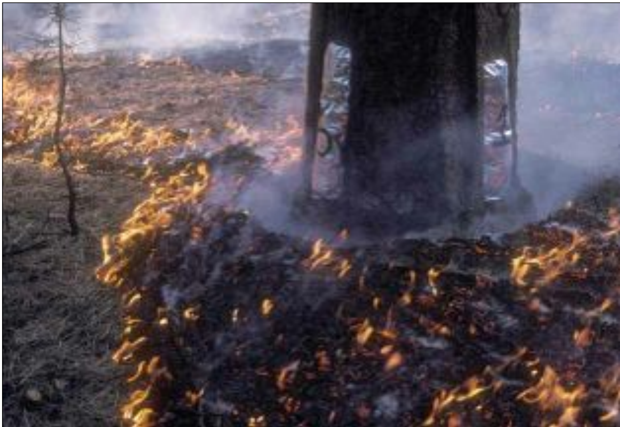
Figure 3. Soil and cambium temperatures being measured during a prescribed fire at Limestone Flats research area where the forest floor material has been removed around the base of the tree.
