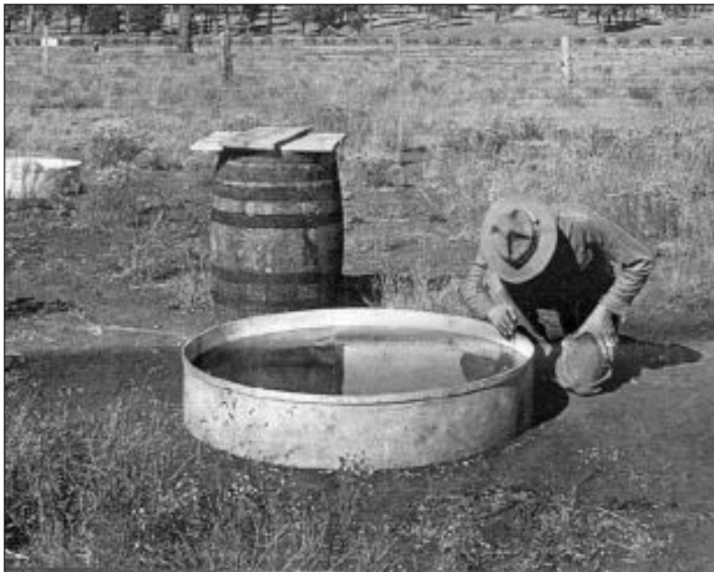
G. A. Pearson measuring water level in evaporation pan. USFS photo 90950 by A. G. Varela, 1912.
