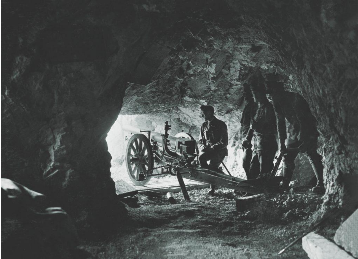
A four-man team of soldiers in an Austrian artillery unit ready an 8cm Feldkanone M.5, the standard field gun of the Austro-Hungarian army in World War I, that's been hidden in the entrance to a cave. (Österreichische Nationalbibliothek) (Österreichische Nationalbibliothek)
