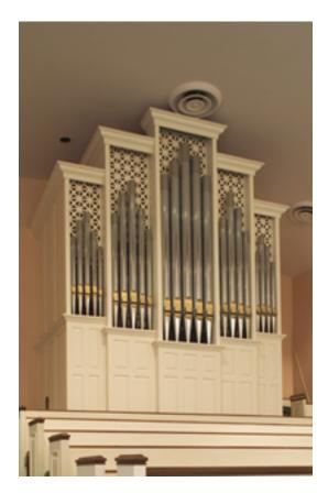
The Antiphonal Organ, whose name suggests its musical role, is comprised of both an unenclosed Principal chorus and an enclosed/expressive "swell" chorus. In addition, this division is fitted with a two-manual and pedal tilting-tablet console capable of controlling the Antiphonal resources or, through "blind" General pistons, the resources of the entire organ.
